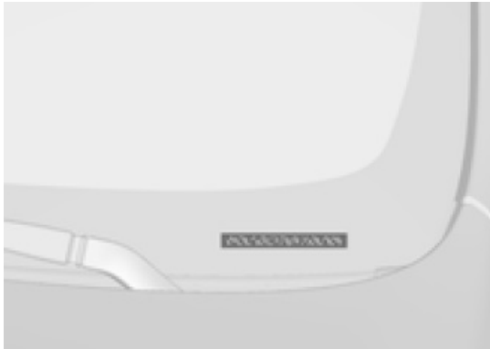
The Vehicle Identification Number is visible through the windscreen.
