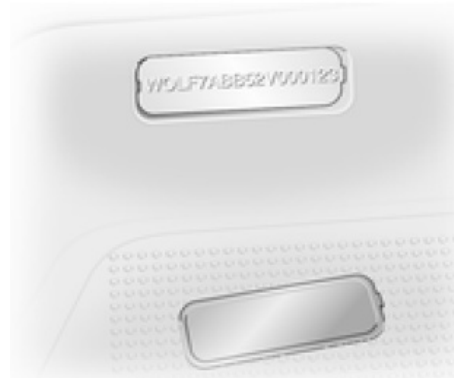
The VIN is also displayed behind a removable plastic cover on the right hand side door step.
